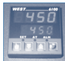
Figure 5 Temperature controller. The upper display is the controlled variable and the lower is the setpoint.
