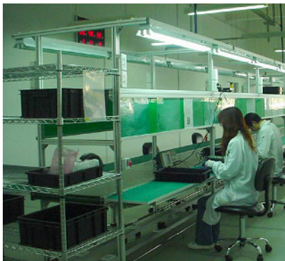
Suzhou workers Cindy and Marty are testing ARCNET transceivers coming down the assembly line.
