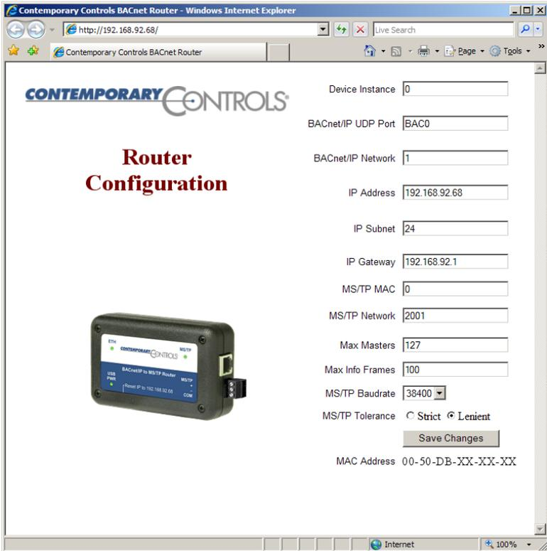
*Figure 10 — Router Configuration Page with Default Values*
