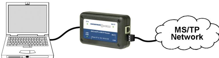
*Figure 8 — Setup for Initial IP Address Configuration*
