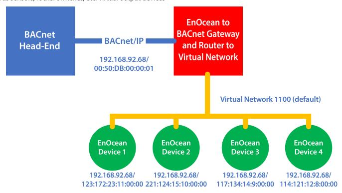
In this image, the BACnet head-end sees the EnOcean devices as standard BACnet devices through the EnOcean to BACnet Gateway, which acts as a BACnet router to the virtual network containing the EnOcean devices. Each EnOcean device has the IP address of the gateway and appears to be on network 1100 with an automatic BACnet MAC address.
