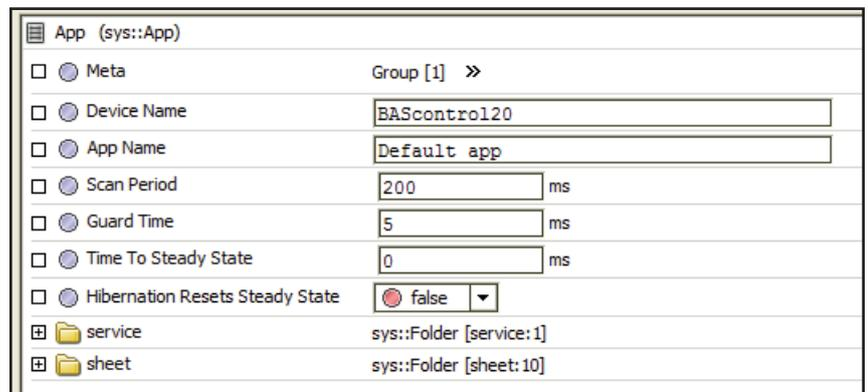
There are two ways to reach the wire sheet. The first is just to click on the **sheet** folder in the App property sheet. The second is to go to the Navigation pane and expand the navigation tree for the controller being accessed. By clicking on **sheet**, you should be able to see the main wire sheet although the default wire sheet is blank.
