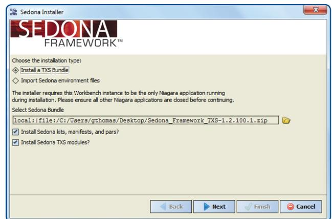
Go to the Contemporary Controls' web site and click on **Support > Product Support Materials > Sedona** and download the Sedona Framework TXS Bundle for either Workbench 3.7 or 3.8 to match the Workbench version you have. The Workbench version is clearly marked on its welcome screen.
