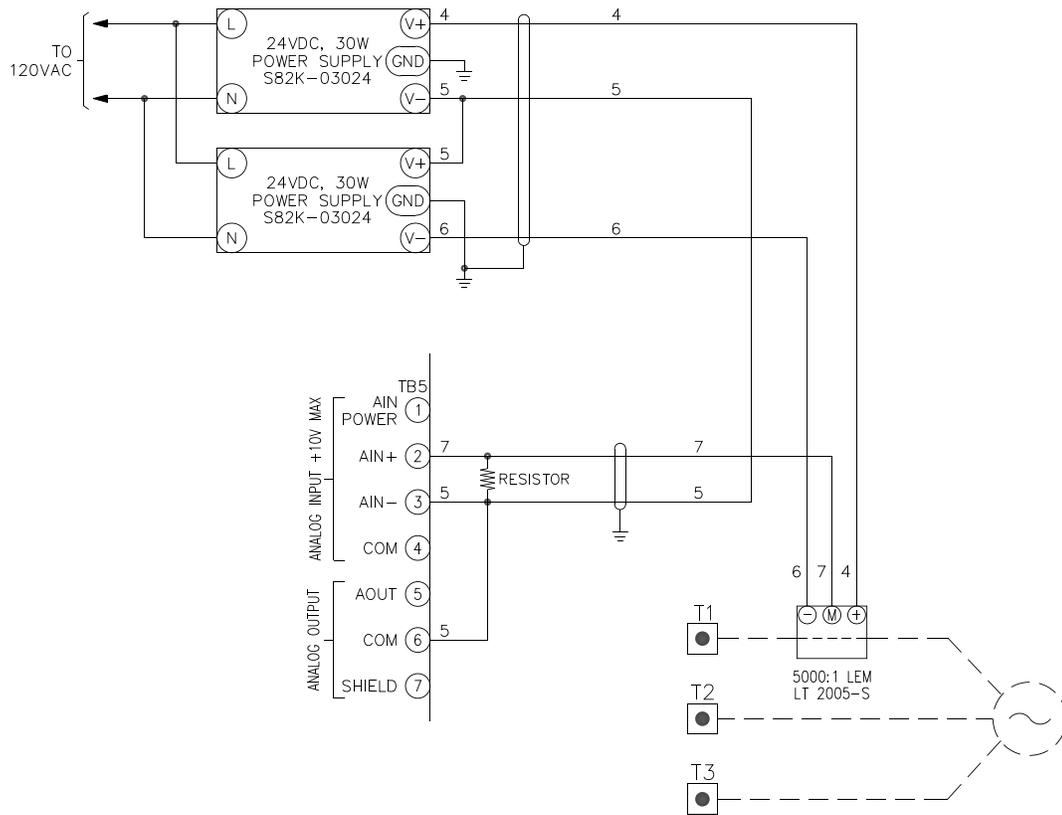
⚠ **NOTE:** Hall effect current sensor must be used when load inertia exceeds motor manufactures recommended specifications.
