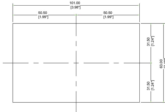
**Figure 20: Large Display Keypad Mounting Dimensions**
