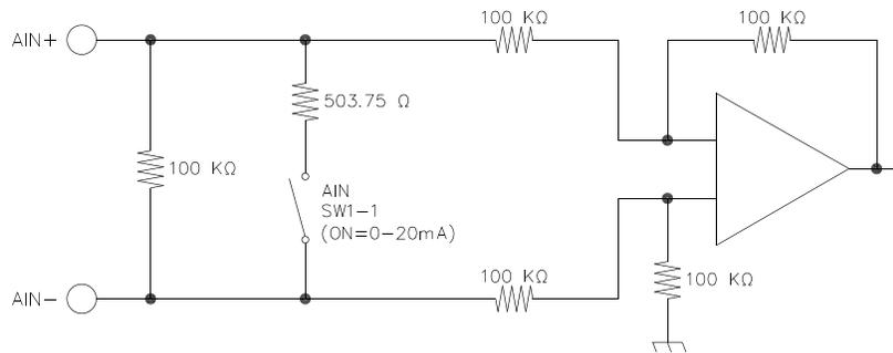
**Figure 50: Analog Output Simplified Schematic**
