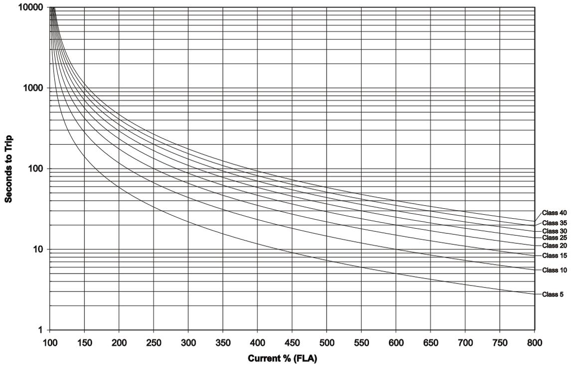
⚠ **NOTE:** In some cases the power stack rating may determine what motor overload settings are available. Each power stack is designed to support specific motor overload classes. The RB2 power stack is designed for class 10 duty without derating. Refer to the RB2 for the specific RB2 overload capabilities. Also, in certain heavy duty DC braking applications, the overload settings may be limited to protect the motor from potential damage during braking.
