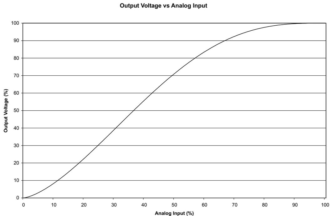
A reference input value of 0% results in no output. A reference input value of 100% results in full (100%) output voltage. The actual input voltage / current that results in a given output can be adjusted through the use of the Analog Input Offset and the Analog Input Span parameters.
