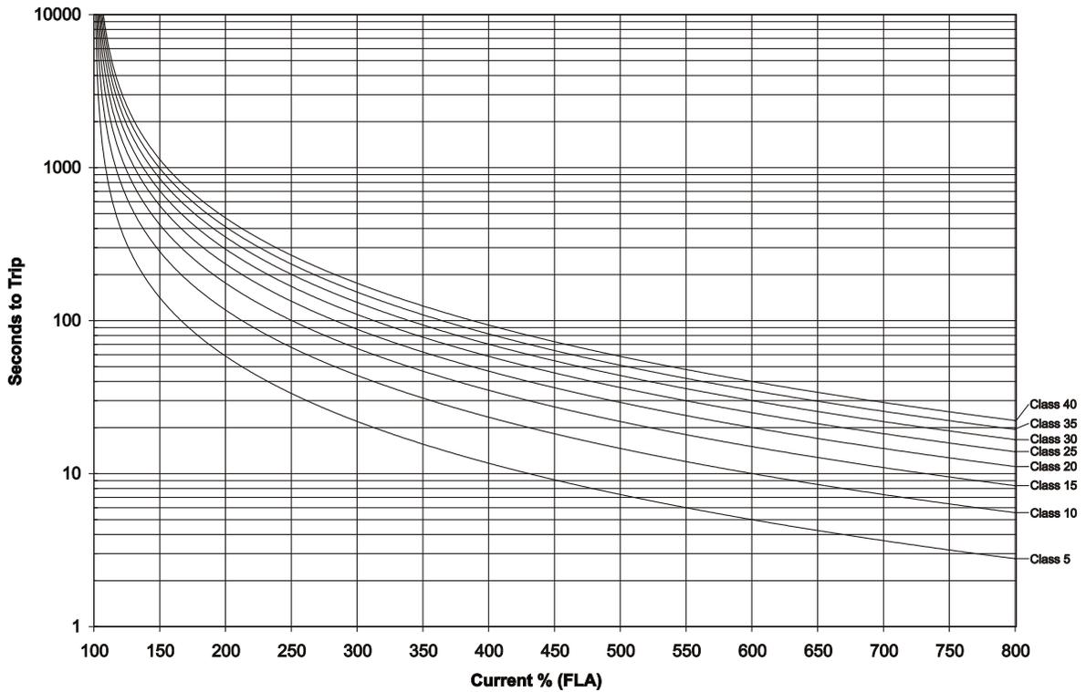
The motor overload will NOT trip when the current is less than motor Full Load Amps (FLA) \* Service Factor (SF).
