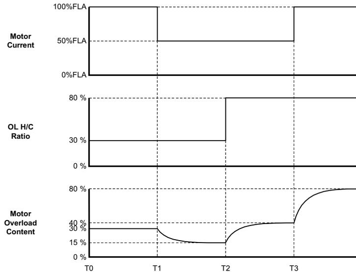
At time T0, the motor current is 100%FLA and the OL H<sup>o</sup>/C Ratio is set at 30%. It is assumed that the motor has been running for some time and the motor overload content has reached a steady state value of 30% (30% H<sup>o</sup>/C Ratio x 100% FLA = 30%).
