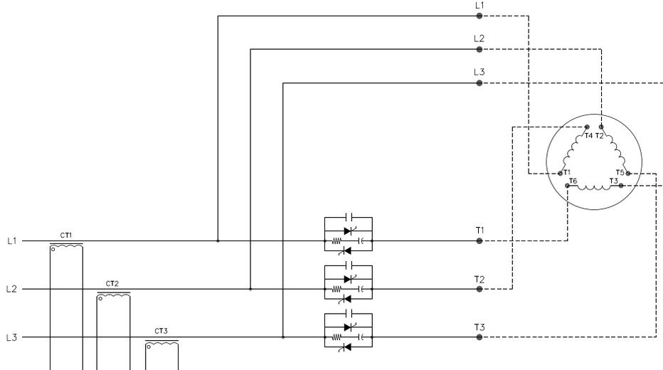
For an inside delta connected motor, the starter current is less than the line current by a factor of 1.55 (FLA/1.55). By comparison of Figure 39 and Figure 40, the most obvious advantage of the inside delta starter is the reduction of current seen by the soft starter. The soft starter can be downsized by a factor of 1.55, providing significant savings in cost and size of the starter.
