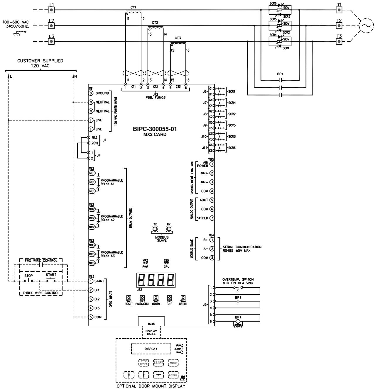
Figure 9: Power Schematic for RB2 High HP
