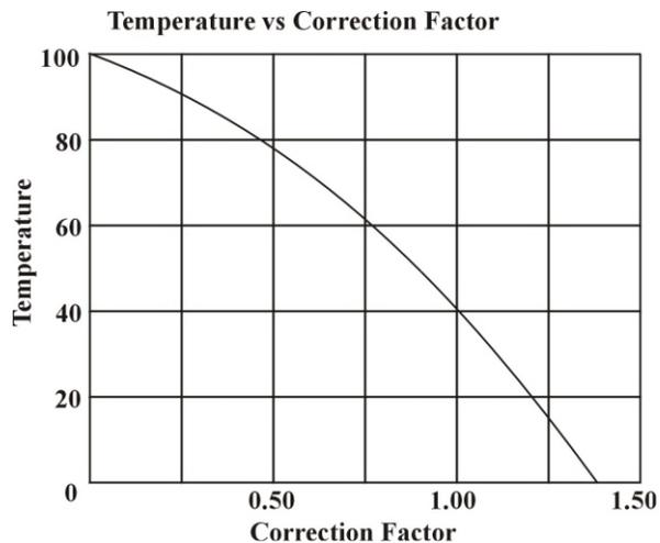
Example: If a motor operates at 0°C, then a 1.36 correction factor could be applied to the overload multiplier. This could give a theoretical overload multiplier of 1.36 x 1.25 or 1.70. The highest legal NEC approved value of overload multiplier is 1.40, so this could be used.
