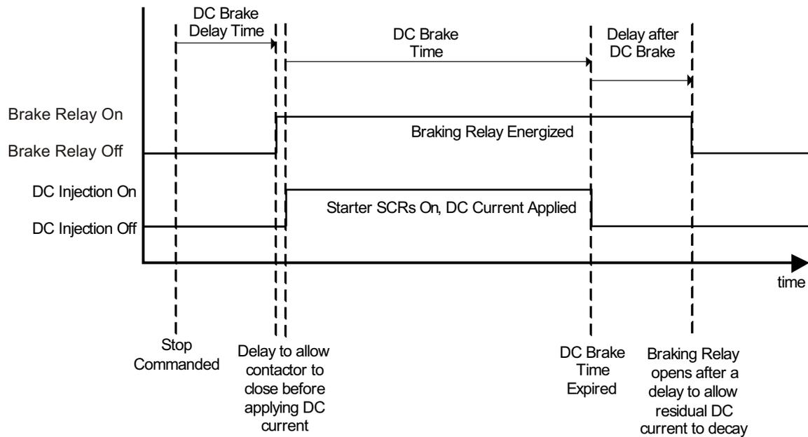
After the DC Brake Time has expired, the Braking Relay is held energized to allow the DC current to decay before opening the freewheel path. This delay prevents a contactor (if used) from having to open significant DC current which greatly prolongs the life of the contactor. This delay time is based on motor FLA, the larger the motor the longer the delay time. The delay after DC brake time is approximately:
