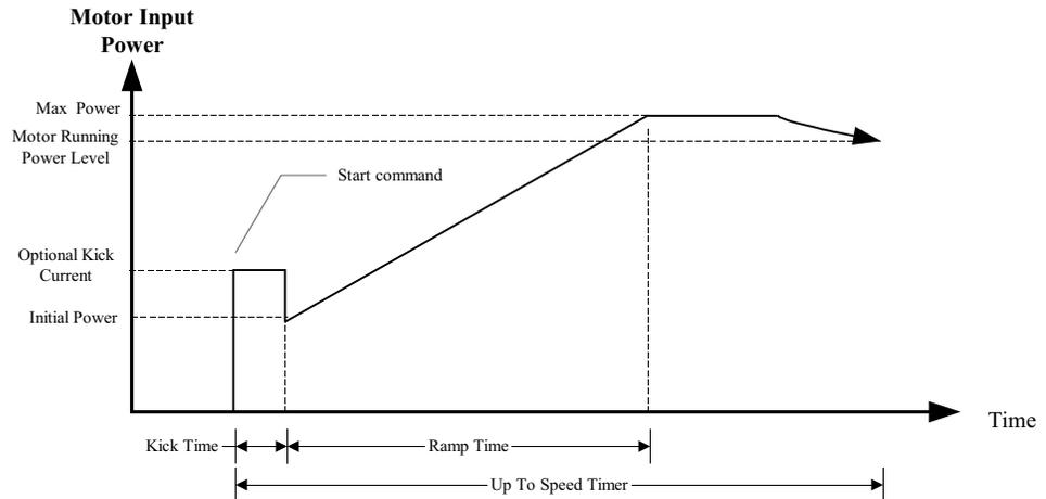
Power control acceleration can be very useful for a variety of applications. Power control generally should not be used in applications where the starting load varies greatly during the start such as with a reciprocating compressor. Power control is not recommended for starting of AC synchronous motors.
