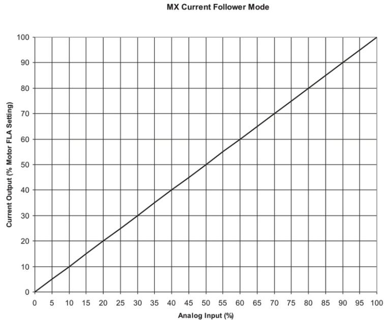
A reference input value of 0% results in no output. A reference input value of 100% results in a current output equal to the Motor FLA setting. The actual voltage or current input that results in a given output can be adjusted through the use of the Analog Input Offset and Analog Input Span parameters.
