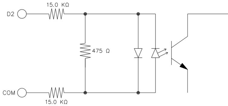
**Figure 49: Analog Input Simplified Schematic**
