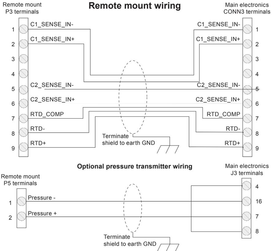
**Fig. 28 Remote mount wiring**
