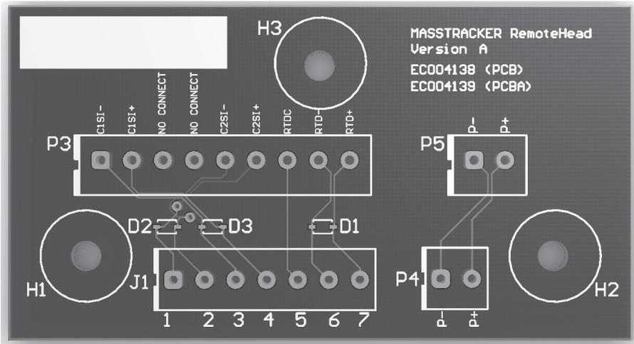
**Fig. 29 RIM10 remote mount PCBA**
