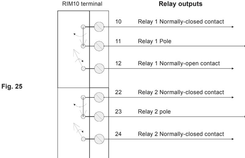
An alternate view of the relay contacts is shown below:
