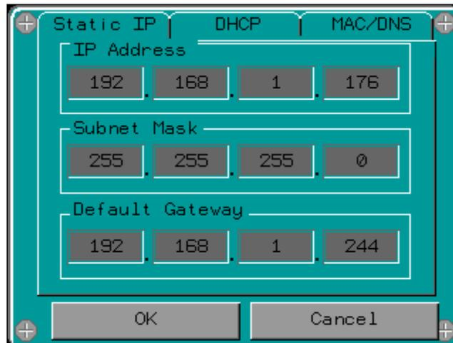
The network settings screen allows the IP address to be changed. When complete, press **OK**. When returned to the HMI system configuration page, press **To Run Mode** to apply the changes. Press **OK** when prompted to reboot the HMI with the new IP address settings.
